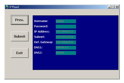
This page shows the information of the selected device to check if there is any mistake or not. If it is correct, please press "Submit" button and the setting information will be uploaded to the selected device. Click on "Exit" button if you don't want to set it up; Click on "Prev." button to go back to the previous page for the modification.
